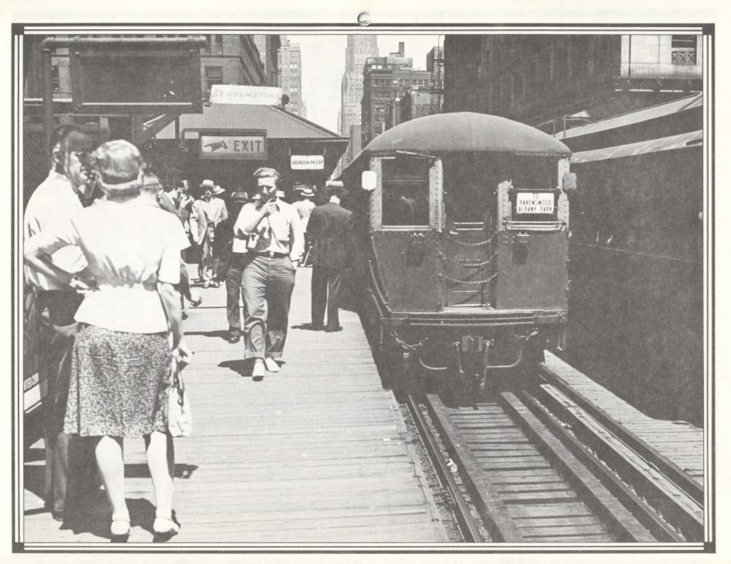
Before the State Street subway was opened in 1943, all trains from the North Side entered downtown on the Outer Loop. Semi-remote door controls adorn the front of this all-steel Ravenswood train at Quincy. Marker lights and a portable headlight were attached only for night service.
