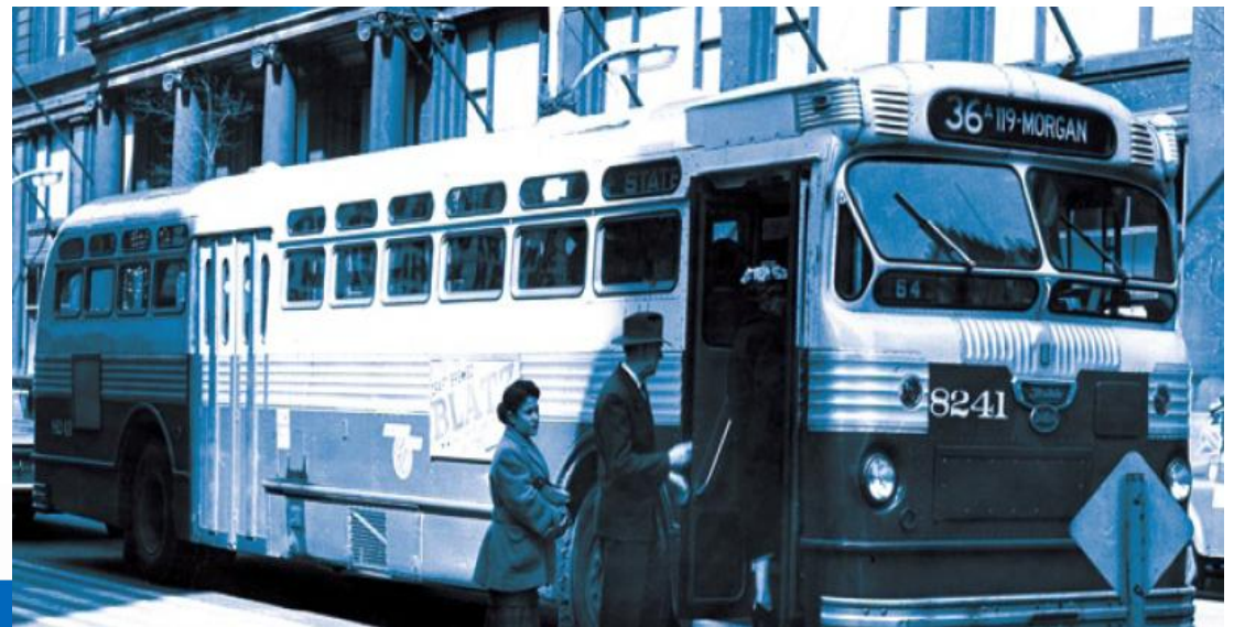
The 1958 Flexible propane powered bus
